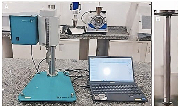
Figure 1. Photographic image of the penetrometer connected to the laptop (A) and the conical tip penetration probe with a 30° angle and 12.37 mm 2 base area.
